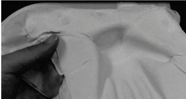
Figure 6. Deformation of fabric-jamming sheet. This image shows a fabric-jamming sheet obtained by evacuating the inner air after deforming with hand.
